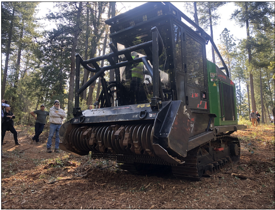
NATALIE HANSON — ENTERPRISE-RECORD Bobcat Chico's machine for mastication, turning trees to mulch, for fire prevention is demonstrated Friday in Cohasset.
