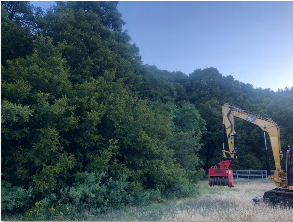
Figure 56. Excavator with masticator attachment.
