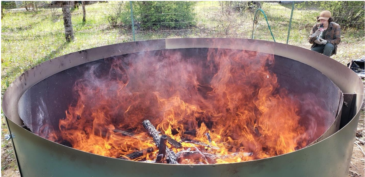
Figure 5. The Ring of Fire Kiln from Wilson Biochar can make a cubic yard of biochar in about 4 hours.
