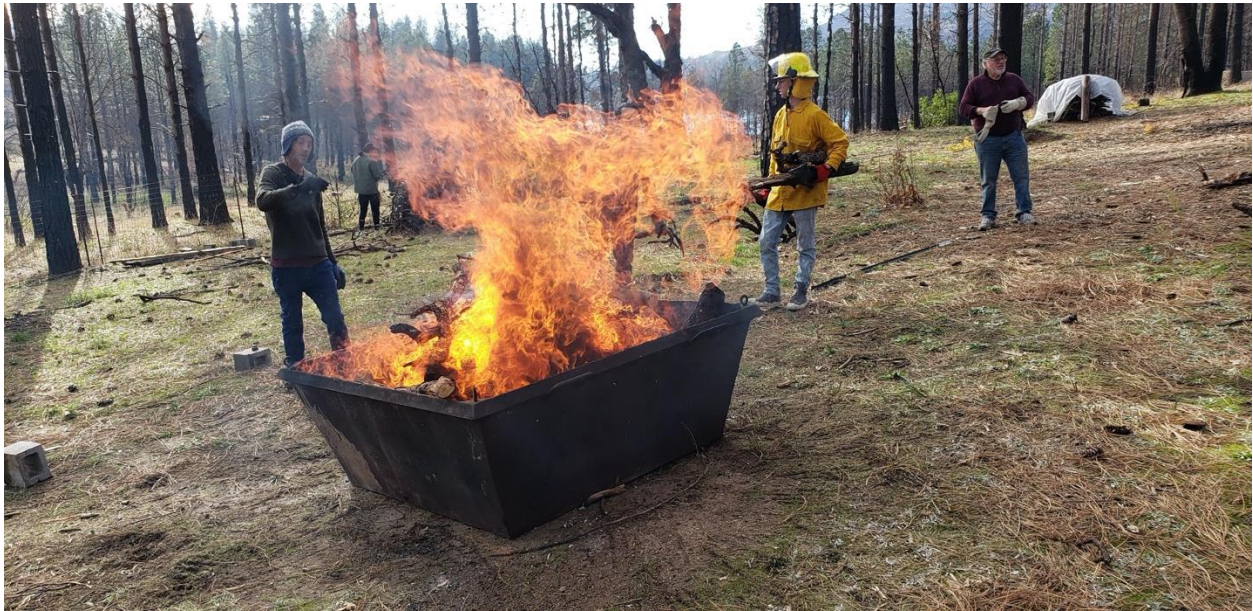
Figure 1 Forest workers make biochar in a kiln on a property in Paradise, CA in January 2020.
